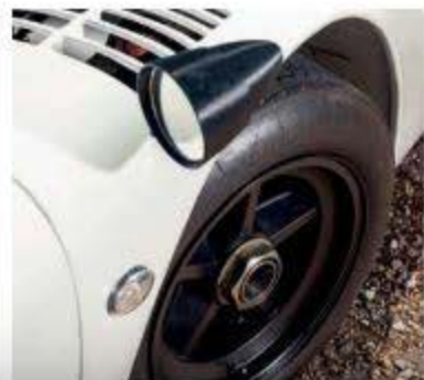
Left Wheels are custom recreations made from a 3D model of an original 917 five-spoke
